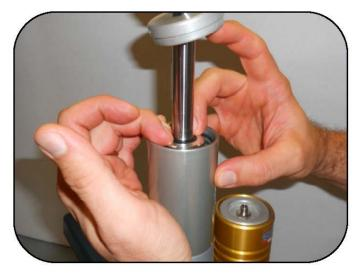
Press down on the shaft guide to expose the snap ring.
