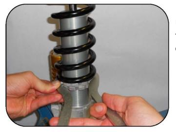
Using 2 wrenches (00529000087), tighten the preload ring against the counter preload ring.
