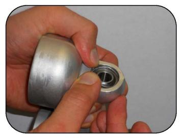
Install the snap ring making sure it is seated the entire circumference of the groove.
