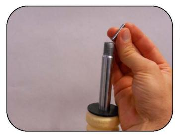
Install the shorter steel adjustment rod.
