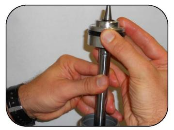
Keeping the shaft position fixed, slide the guide onto the shaft observing the orientation in the photo. .
