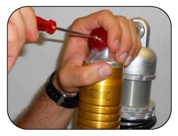
Turn the low speed adjuster all the way in and then back out the number of clicks recorded before removal.The factory setting is:20 clicks out on the 2T22 clicks out on the 4T.
