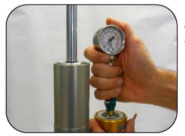
Check the pressure with a reliable and calibrated gauge.
