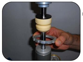
Remove the counter preload ring.
