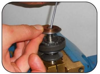
Remove the rebound valve stack of shims.
