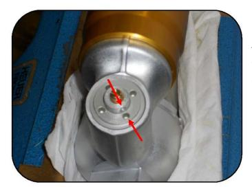
Align the locking hole of the knob with one of the 4 holes on the compression assembly. Note the arrows in the photo.
