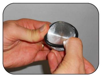
Install the outer diaphragm O-ring.
