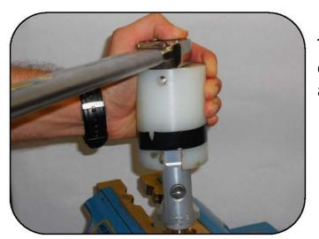
Tighten to 70Nm using the shock clevis socket bushing (005299000090) and a torque wrench.
