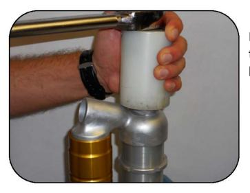
Being careful that the base is hot, loosen the base from the shock body using the base socket bushing tool (005299000088)
