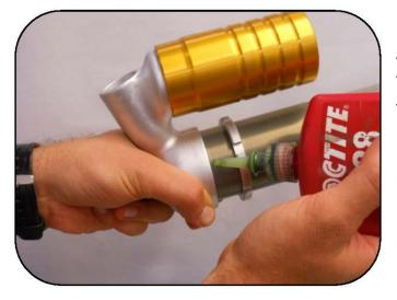
Apply a high strength thread locker to the external threads on the body near the base.
