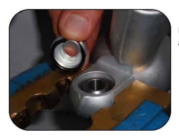
Note: The bushing will be removed along with an O-ring.
