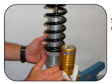
Spin the spring counter preload ring up against the preload ring.
