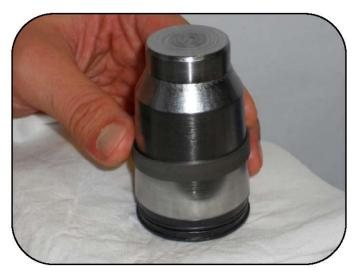
Install the piston Teflon band pushing down firmly using the piston sleeve (005299000092).
