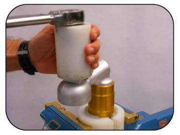
Secure the tank in a vise using the shock body plastic jaws (00529000089) Tighten the base using the base socket bushing (00529000088) and torque to 50Nm.
