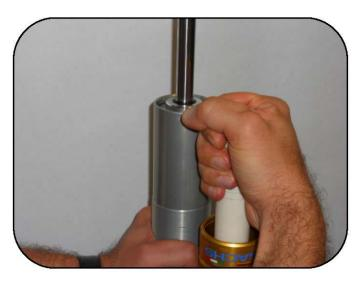
Push the diaphragm all the way down, the shaft should rise.
