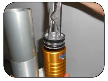
Using reverse needle nose pliers or snap ring pliers, remove the separator diaphragm completely from the tank.
