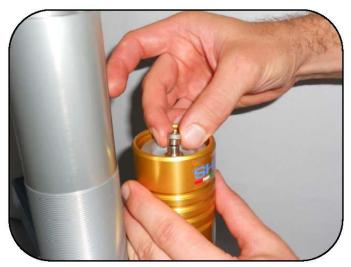
Screw the cap back on the tank valve.
