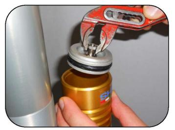
Using pliers, pull up on the tank valve cap until it is removed from the tank.
