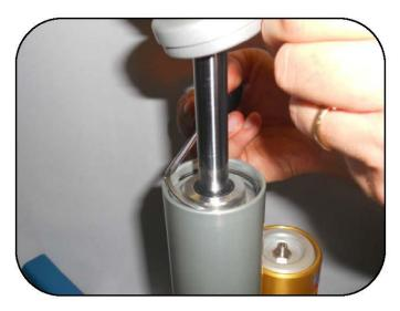
With a screw driver , pry up on the snap ring being careful not to scratch the inner side of the shock body.
