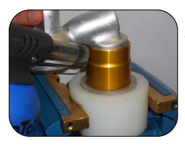
Using the plastic jaws (0052990000898) to secure the reservoir tank, heat the base/tank junction with a torch.
