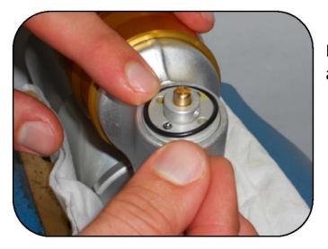
Place the O-ring onto the compression assembly.
