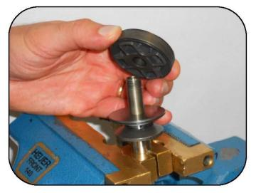
Insert the piston on the shaft making sure the 4 square holes are facing downward.
