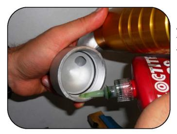
Apply a medium strength thread locker to the entire circumference of the inner threads of the base.
