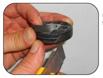
Use a cutter to remove the Teflon band from the piston.
