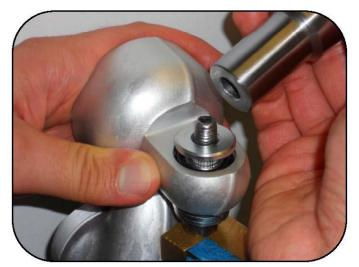
Resting the head of the bolt on the vise, place a metal sleeve over the bolt resting against the flange bushing.
