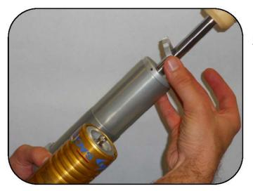
Slide on the spring counter preload ring and screw it down toward the base.
