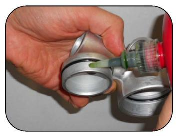
Apply a medium strength thread locker to entire circumference on the threads of the tank side of the base.
