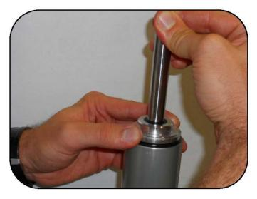
Keeping the shaft position fixed, slowly push the shaft guide into the body until the O-ring starts to seal. A small amount of oil will leak out and this will ensure no air bubbles are trapped under the guide.
