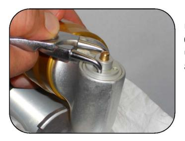
Using the compression nut tool (AVT-0127-002-T01-3)or round nose pliers, unscrew the compression adjuster assembly.
