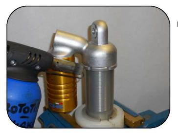
Using a torch, heat the base locking ring.
