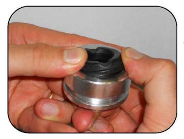
Place the rubber extension limiter into the guide.
