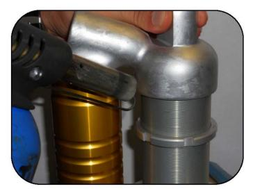
Heat the junction of the base and shock body with a torch.
