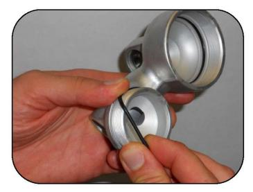
Install the outer O-ring over the tank side of the base making sure it is fully seated.
