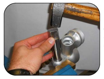
Flip the base and secure in the vise. Using the correct size metal press tool, tap out the uniball. Note: The uniball can only be removed from the side with the snap ring groove.
