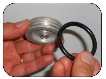
Remove the O-ring form the tank cap.
