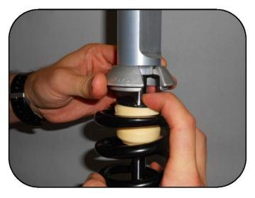
Push down on the rubber bumper to make room to remove the spring collar.
