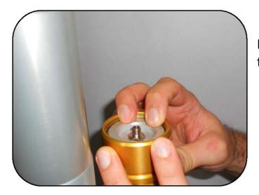
Push down on the reservoir tank cap to expose the snap ring.
