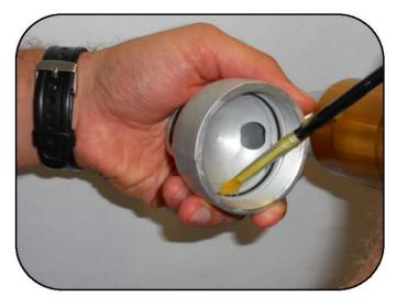
Lightly grease the inner base O-ring area.
