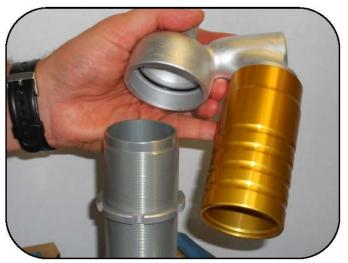
Remove the base form the shock body.
