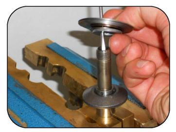
Lock the shaft into the vise using the brass jaws (005299000091), then install the calibrated compression shim stack.
