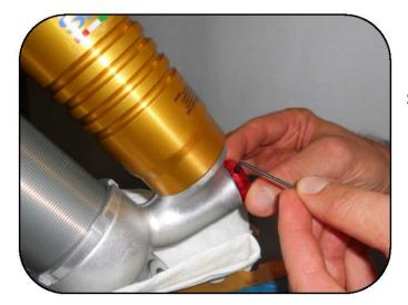
Use an Allen wrench to loosen the high speed compression dial lock nut.
