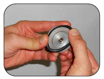
Install the O-ring on the outer edge of the reservoir cap.
