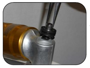
Place the compression valve assembly into the base opening noting the orientation in the photo.
