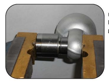
Using a vise, press the uniball into the base from the side that has the snap ring groove.
