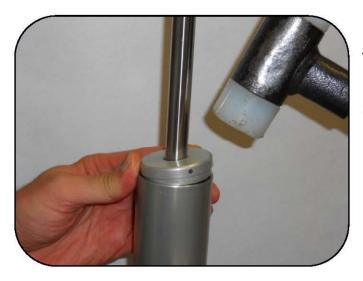
To seat the cap, place it on the shock body and lightly tap around the circumference with a rubber mallet.
