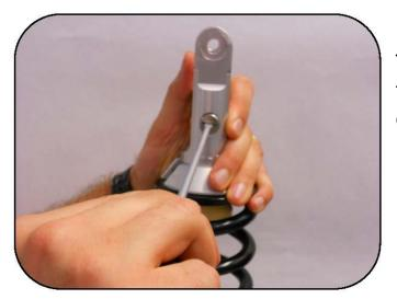
Turn the rebound adjusting screw all the way in then back out the number of clicks recorded before removal. The factory setting is: 20 clicks out for the 2T 18 CLICKS for the 4T.
