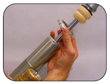
Slide on the spring preload ring keeping the flange pointed up.
