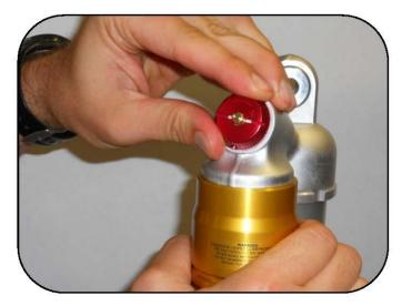
Return the high speed compression dial to the pre removal setting. The factory setting is: 20 clicks out on the 2T 22 clicks out on the 4T.
