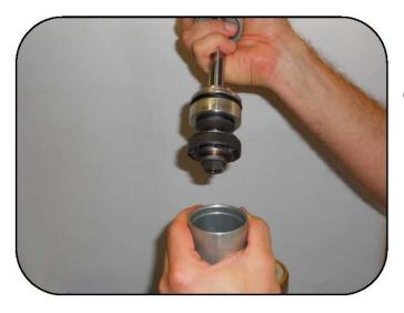
Pull up on the shaft to remove the damper assembly.
