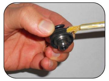
Lightly grease the O-ring on the compression valve assembly.
