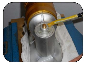
Lightly grease 2 holes opposite each other perpendicular to the locking screw hole.
