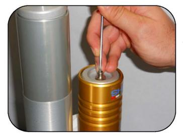
Press the center of the valve to release all pressure from the tank.
