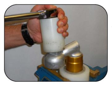
Being careful that the base is hot, using the socket bushing tool (005299000088) loosen the base from the tank.
