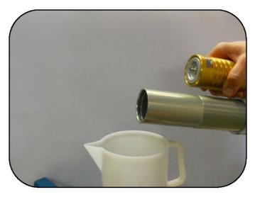
Drain the oil from the shock body.
