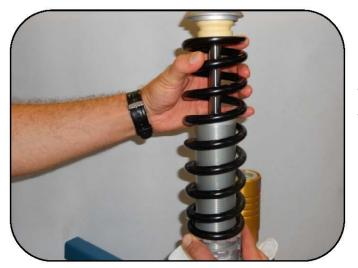
Unscrew the preload ring far enough to reveal the rubber bumper over the top of the spring.
