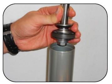
Insert the piston into the shock body.
