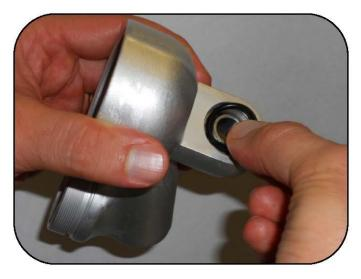
Place the O-ring on the face of the uniball. The grease will help to hold the O-ring in place.
