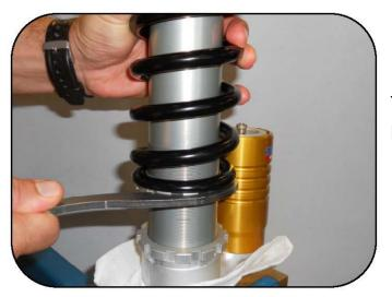
Unscrew the next ring towards the base to completely remove the spring preload.
