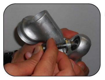
Insert the flange bushing using a bolt.
