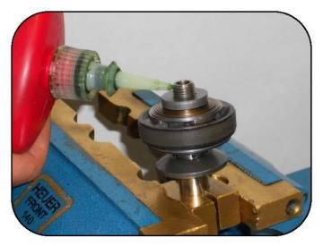
Put a drop of high strength thread locker onto the shaft threads.
