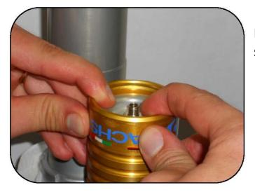
Push the cap in enough to expose the snap ring seat.
