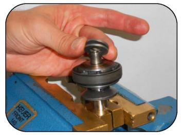
Place the 2 spacers onto the shaft.
