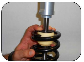
Slide the plastic washer and bumper down to make room for the spring support collar.
