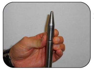
Apply the shaft sleeve to the end of the shaft. (005299000093)
