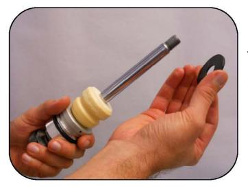
Remove the bumper support washer from the shaft.
