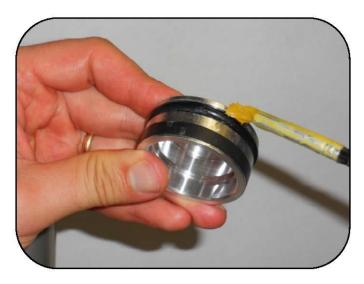
Using Nitrile O-ring grease, apply to the circumference of the O-ring.
