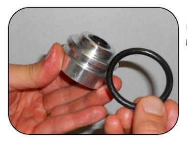
Remove the outer O-ring from the shaft guide.
