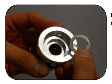
Remove the oil seal support washer from the guide.
