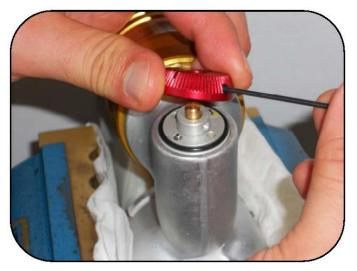
Place the compression adjuster knob on the assembly being sure to align the locking screw with the locking hole on the assembly.
