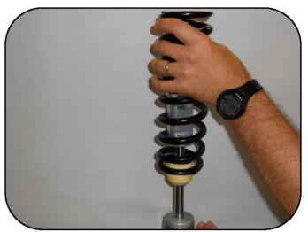
With the spring collar removed, you can now raise the spring off the shock.
