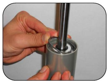
Insert the guide snap lock ring into the seat making sure it is installed completely.
