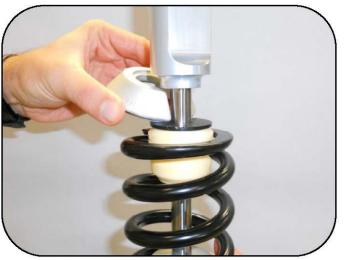
With the rubber bumper out of the way, lower and slide out the spring support collar.
