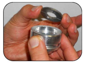
Insert the guide washer making sure the 4 groves are facing down toward the seal.
