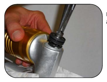
Remove the compression valve assembly.
