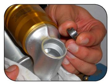
Remove the spring guide bushing.
