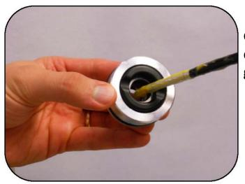
Grease the guide shaft seal circumference with Nitrile rubber O-ring grease .
