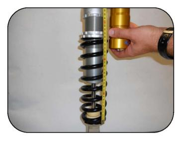
Measure and record the length of the spring under preload.
