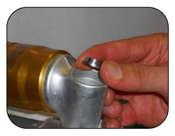
Insert the spring guide bushing observing the orientation in the photo.
