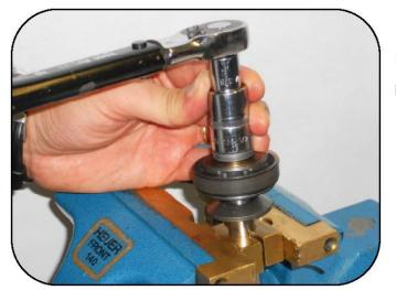
Using a torque wrench, tighten the nut to 40Nm.
