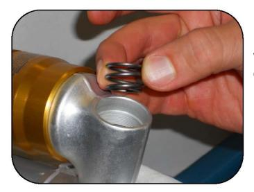
Place the conical spring in the opening with smaller diameter facing downwards.
