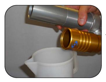
Drain the oil from the tank/shock body. Make sure it is drained completely. This can take a few minutes.
