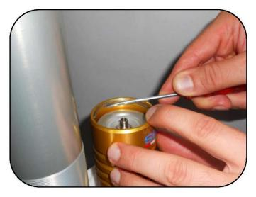
With a screw driver, pry up on the tank snap ring being careful not to scratch the inner side of the tank.
