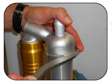
Being careful that the base is hot, use the spanner wrench (005299000087) to loosen the lock ring.
