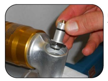
Insert the compression assembly into the base.
