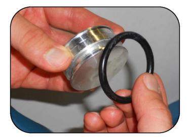
Remove the O-ring from the diaphragm separator.
