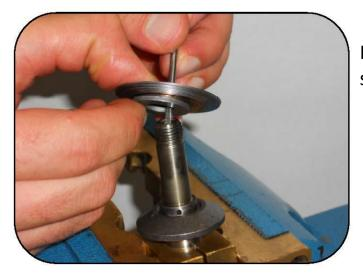
Remove the compression valve stack of shims.
