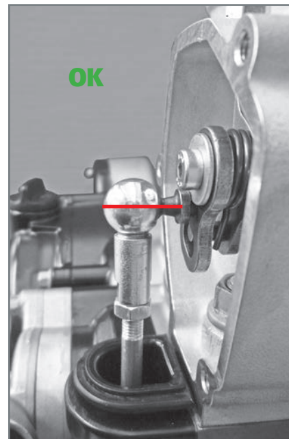
Correct position of the control rod seat.
