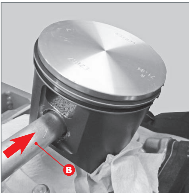
Removal of pin bolt.
