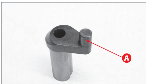
Check of centrifugal control lever A area.
