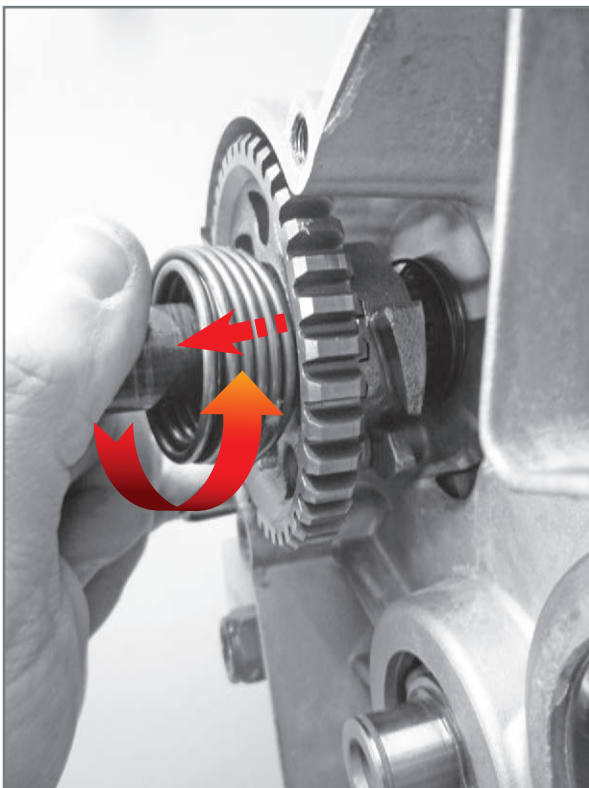
Extraction of shaft from crankcase.
