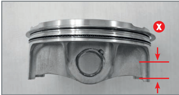
Quota at which to measure the outside diameter of the piston.
