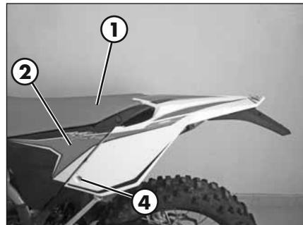
Get off the male end wrenches and hexagon socket **3**. With these is possible to unscrew the screw **4**.
