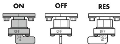
**OFF**: fuel supply closed. Fuel cannot pass from the tank to the carburettor.
