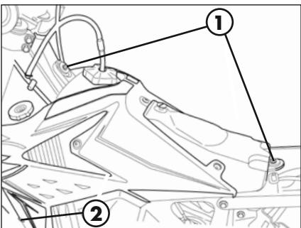
Remove the two screws **1** fastening the tank to the frame and the screw **2** (one per side) securing the fairing to the radiator.
