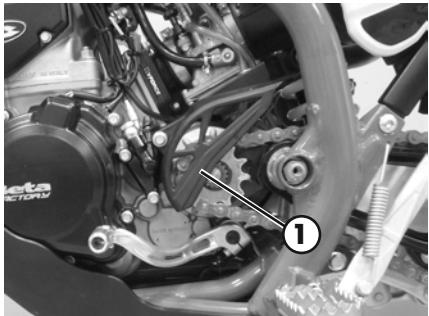
Remove the chain protection **1**, close the tank tap and put a cloth under the carburettor, so that you can collect the running out fuel.
