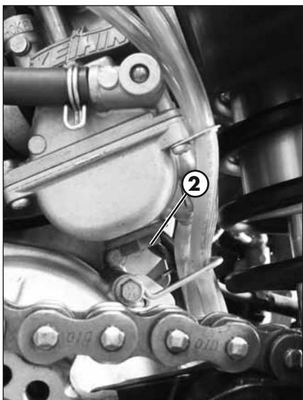
Open the drain screw **2** to drain the fuel.
