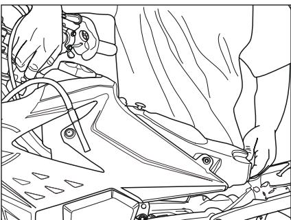
Lift the tank complete with side panels.
