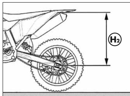
Verify that the value of the static compression  $X = H_1 - H_2$  matches the one shown on page 12. Otherwise, perform the adjustment of the spring preload as described above.
