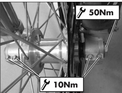
Tighten the wheel bolt and the screws of the foot-leg.
