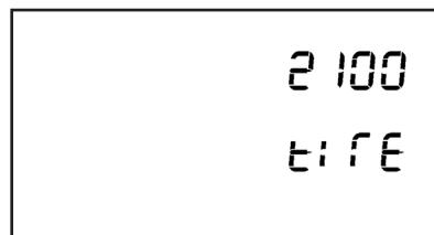
Pushing mode and set more than 2 seconds wheel length is saved. "Saved" will be displayed during 1 second on Dashboard.
