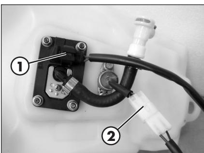
Disconnect the electrical connector **1** and **2**.
