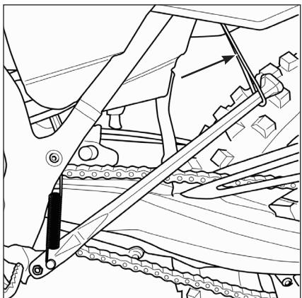
If the vehicle is used off-road, the closed stand can be further fastened by means of rubber band.
