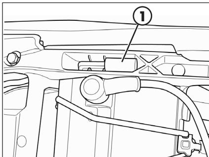
The hex key **1** and its socket wrench (8 mm) are found inside the battery compartment. Remove the seat to reach them (page 80).
