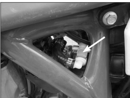
Disconnect the fuel hose by pressing the appropriate button of the quick coupling.
